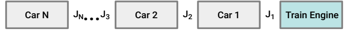
Fig. 1. The train model has a locomotive at one end and N train cars (Car 1, ..., Car N ) coupled with mechanical couplings ( J_1, \dots, J_N ) whose structural integrity must be checked to assert the overall train integrity.
