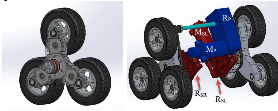
Fig. 9. Detailed design of the locomotion group: a) locomotion unit; b) general arrangement drawing
