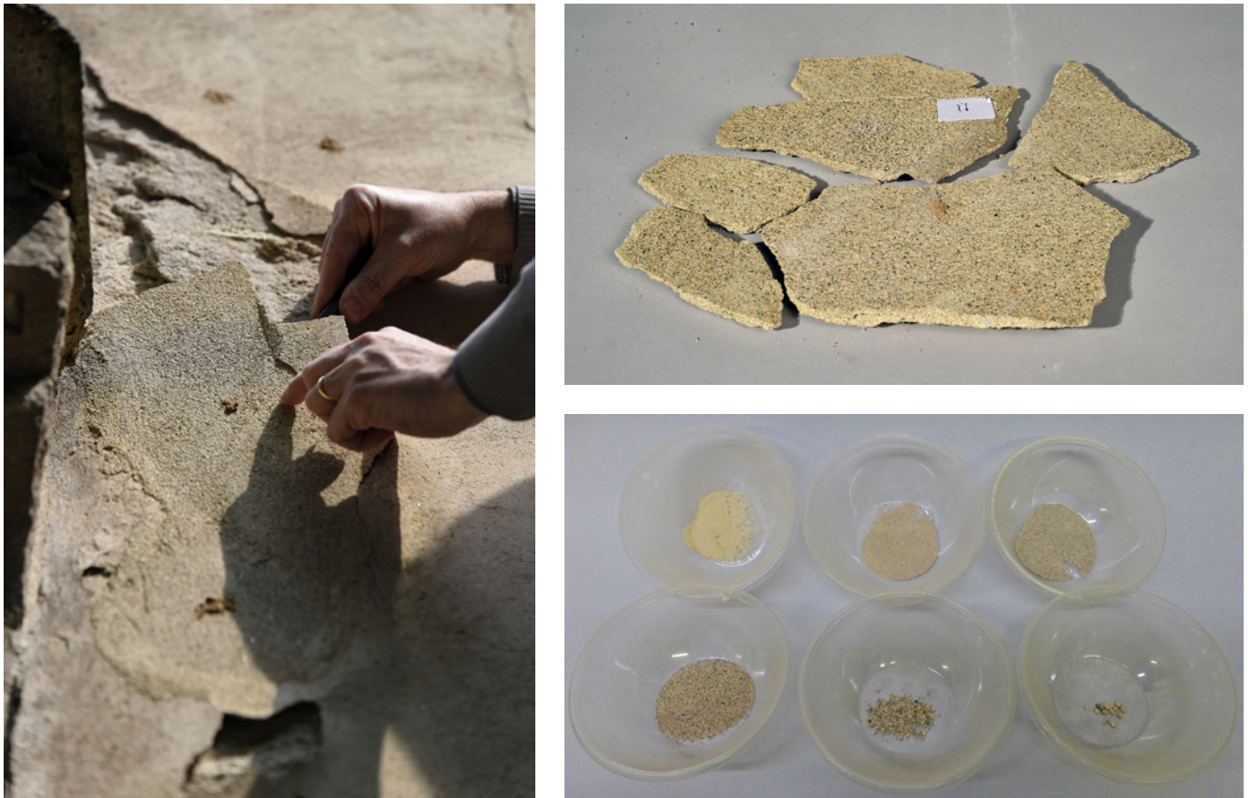
Fig. 1. Serralunga di Crea, Sacro Monte, Chapel 1. A sampling of external render on the south façade (left); Sample 11 (top right); aggregates from disgregation of sample 11 (bottom right).
