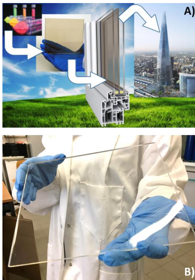
Figure 11. A) The Glass to Power strategy for LSCs to be integrated in smart building; B) Photograph of a Glass to Power panel made of Plexiglass. Adapted and reprinted with permission from [270].
