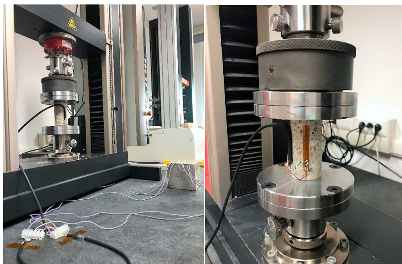
Fig. 2. An experimental set-up for cyclic loading of concrete.
