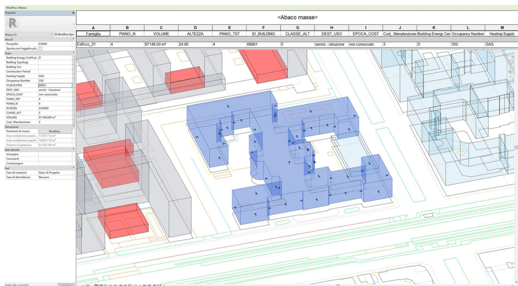
Fig. 2. Geometric and alphanumeric parameters within BIM model.
