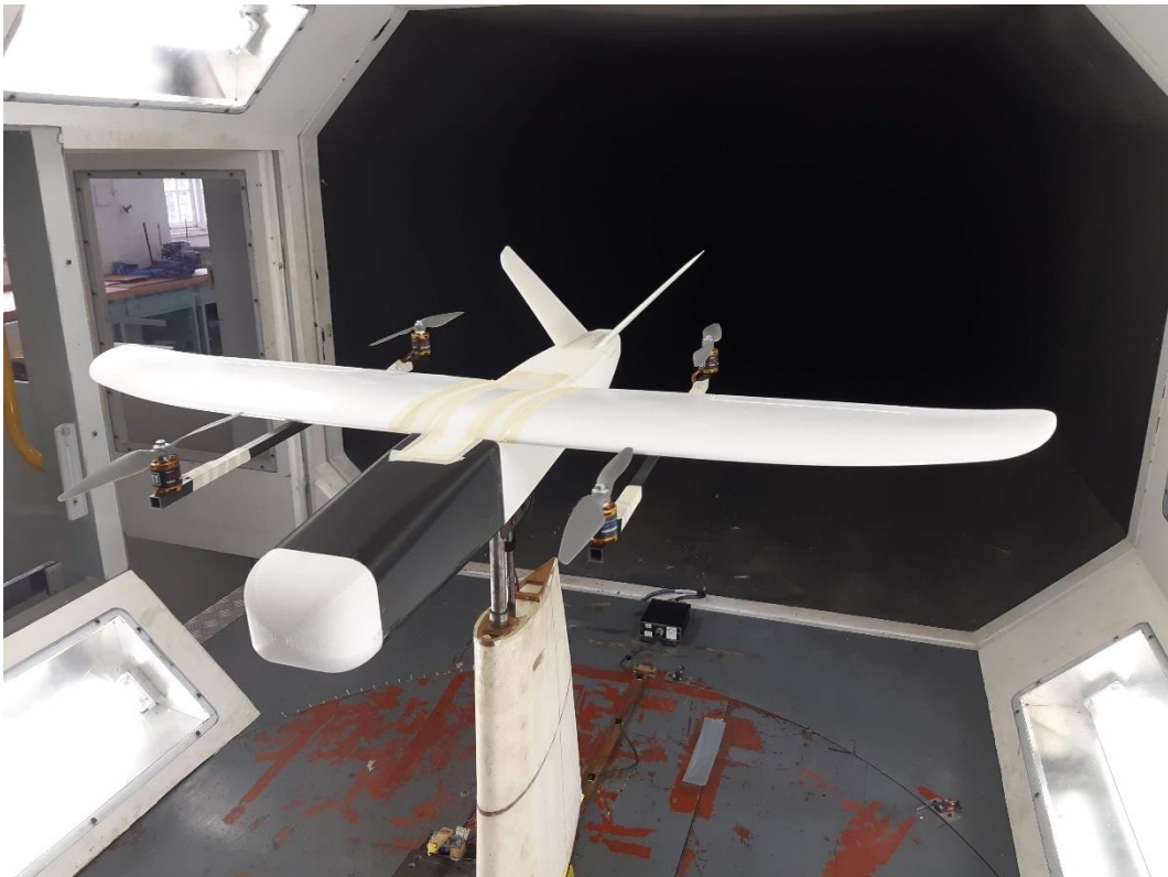
Figure 112: Mini Talon 3, propellers parallel to the airflow.
