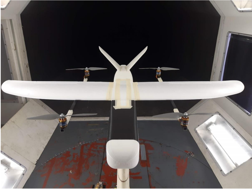
Figure 113: Mini Talon 3, propellers perpendicular to the airflow.
