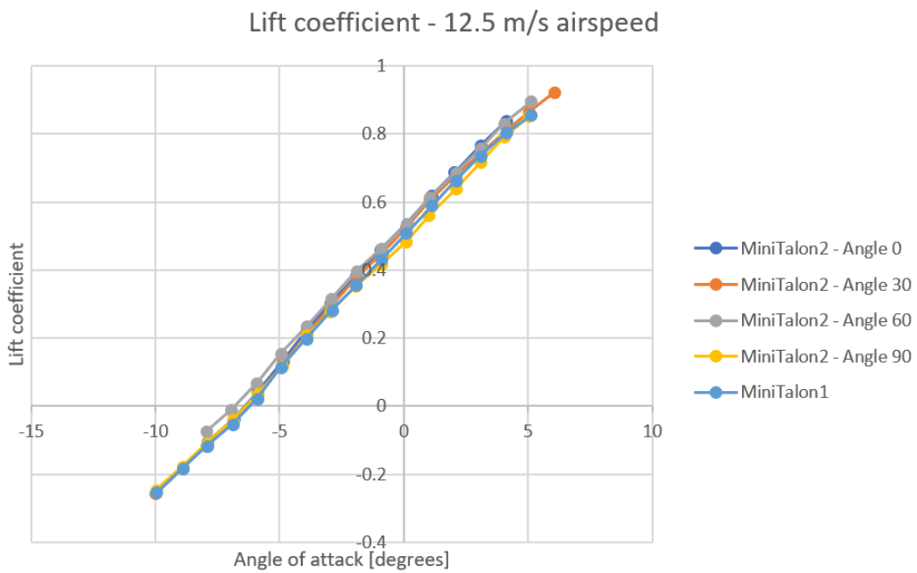
Figure 120: Mini Talon 2, lift coefficient, 12.5 m/s.
