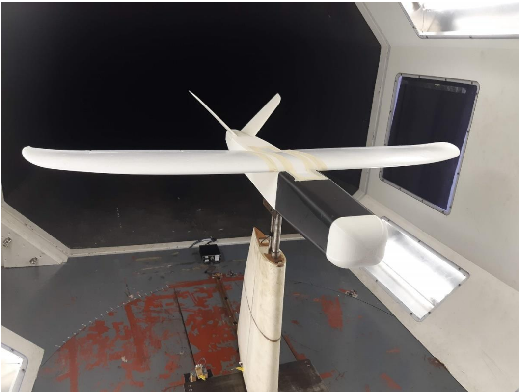
Figure 107: Mini Talon 1 in the University of Sydney 7 by 5 wind tunnel.
