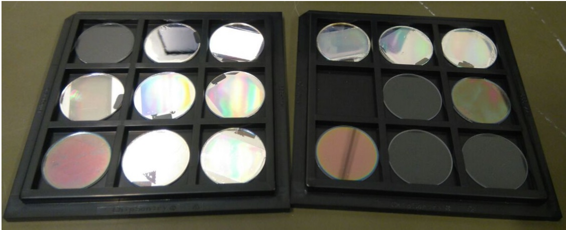
Figure 3.1: The reference and processed glass samples are shown after completing the NIL process for patterning of the diffraction gratings and deposition of the back reflectors.
