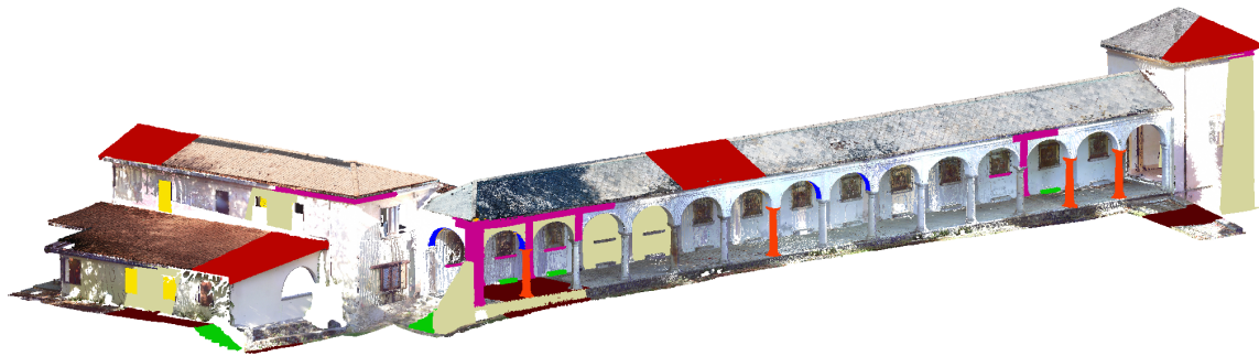
Figure 7. Manual annotations used to train the ML algorithms for the Sacred Mount of Ghiffa (SMG) Scene.
