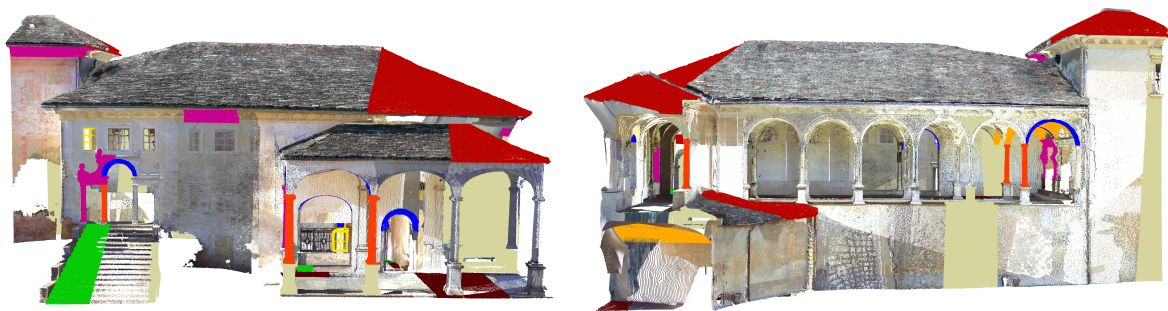
Figure 5. Manual annotations used to train the ML algorithms for the Sacro Monte Varallo (SMV) Scene.
