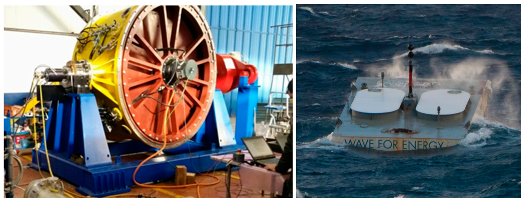
Figure 7. The gyroscopic unit (left) and the ISWEC 100 kW deployed at Pantelleria (right).
