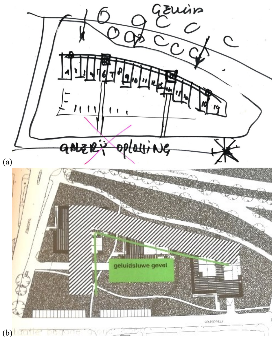
Figure 9.7 – (a) drawing produced by the architect to explain the concept of “gallery” building. Arrows in the upper part indicate the main direction of road traffic noise [=Geluid]; (b) “Possible building form for creating a low-noise façade” as reported in the report from the acoustic consultant
