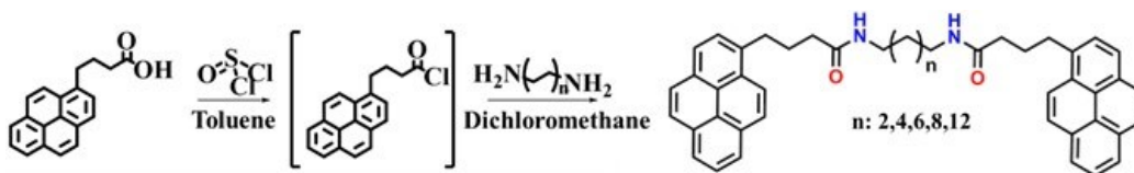
Figure 29. Schematic representation of bispyrene molecules synthesis
