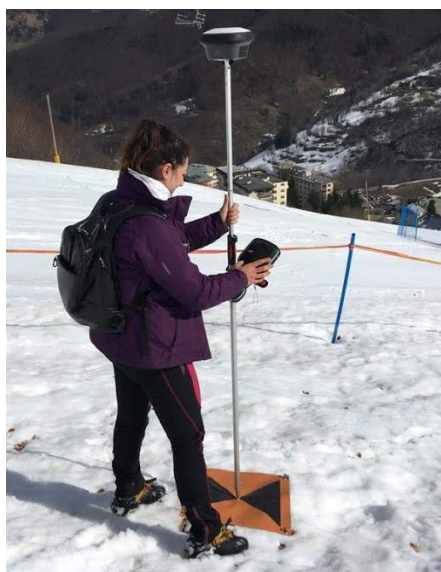
Figure 4. GCPs measurement with RTK approach.
