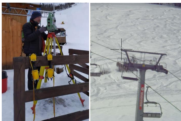
Figure 5. Detail survey with the total station.
