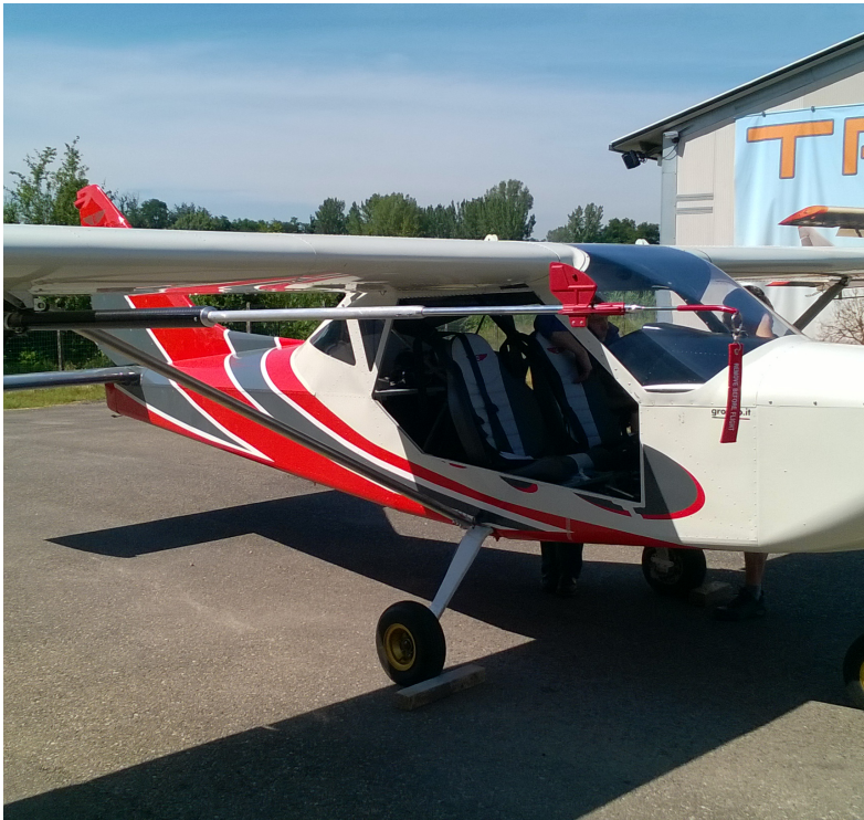
Figure 3.1: Picture of the test vehicle G70 with the AOA/AOS boom mounted under the right half-wing
