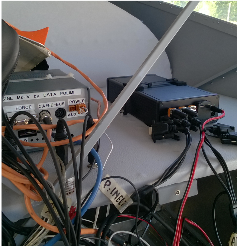
Figure 3.4: Installation of Mnemosine (on the left) and Smart-ADAHRS (on the right)
