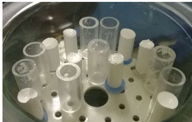
Figure 3-7: Wet HA gelcast dense samples after demoulding.
