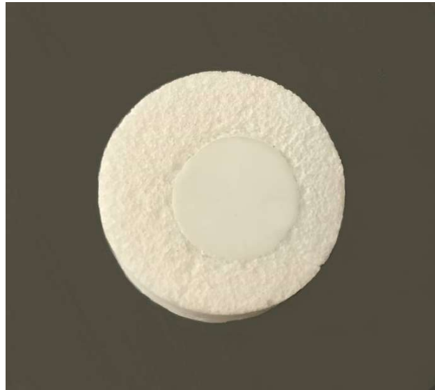
Figure 4-21: Bi-layer sample produced from WBM powder.
