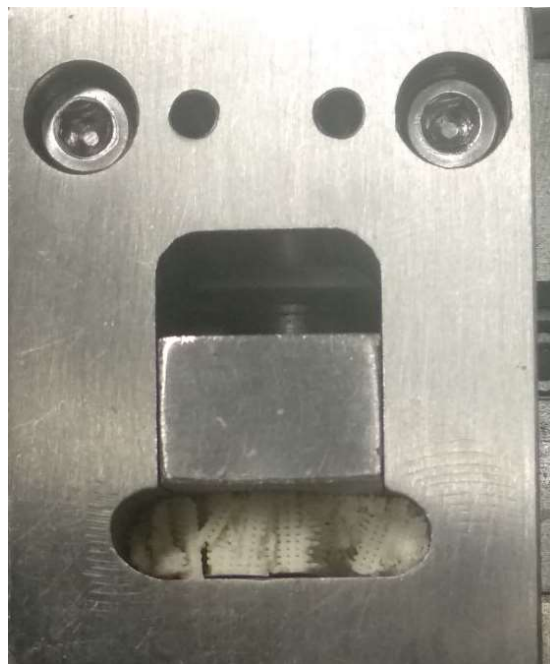
Figure 5-25: Remaining columnar parts of a 3-D porous structure in the sample chamber after unloading of the compression test.
