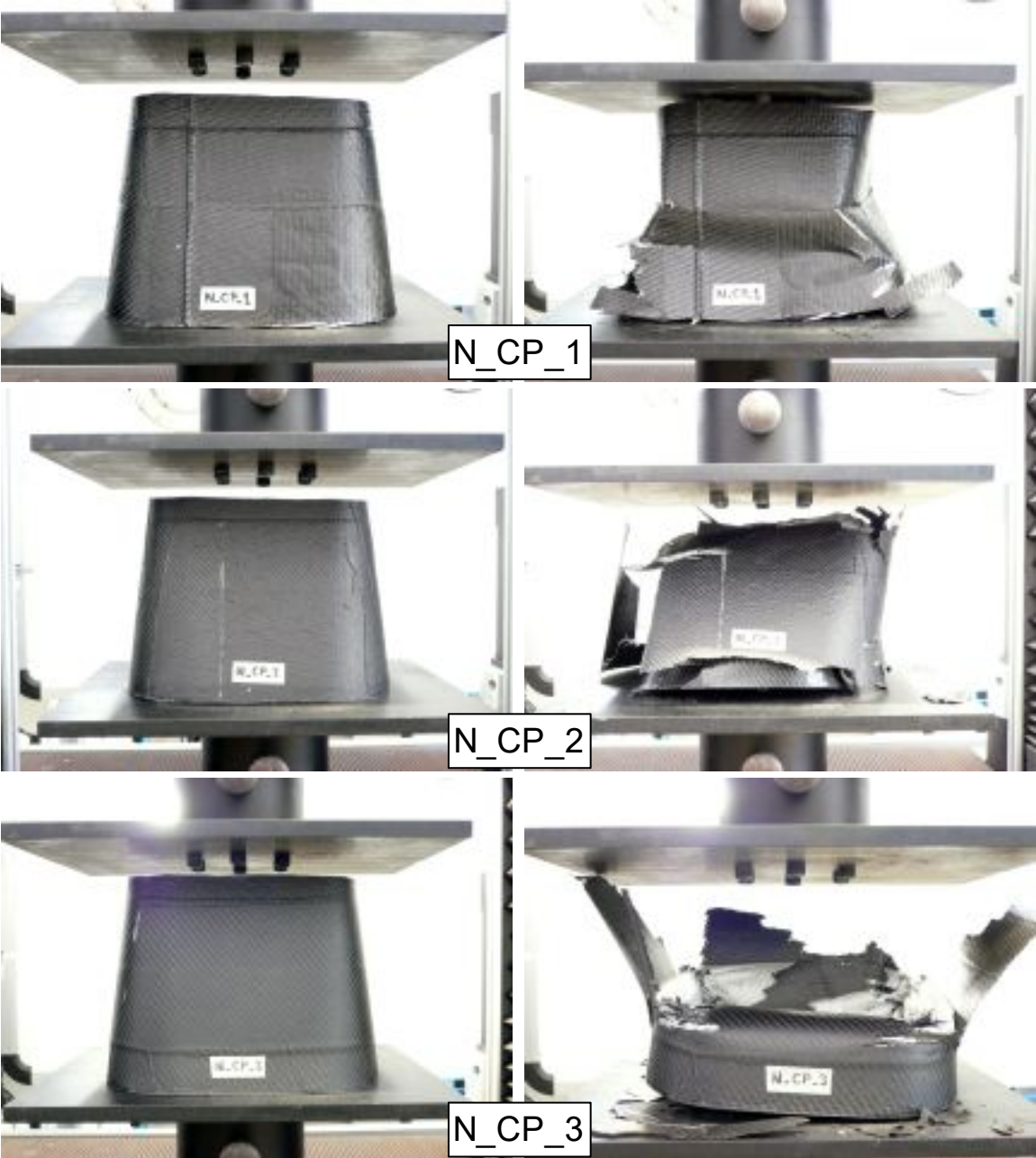
Figure 8: Crushing behaviour of the impact attenuators made of hybrid solution: on the left-hand side the specimens before the tests, on the right-hand side the specimens after the tests.
