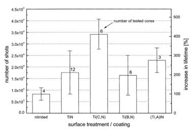
Figure 1.Number of shots achieved in aluminum pressure dies casting for cores of oil pump housing for nitriding and different PECVD coatings. The end of the lifetime is determined by insufficient surface quality of the casting.
