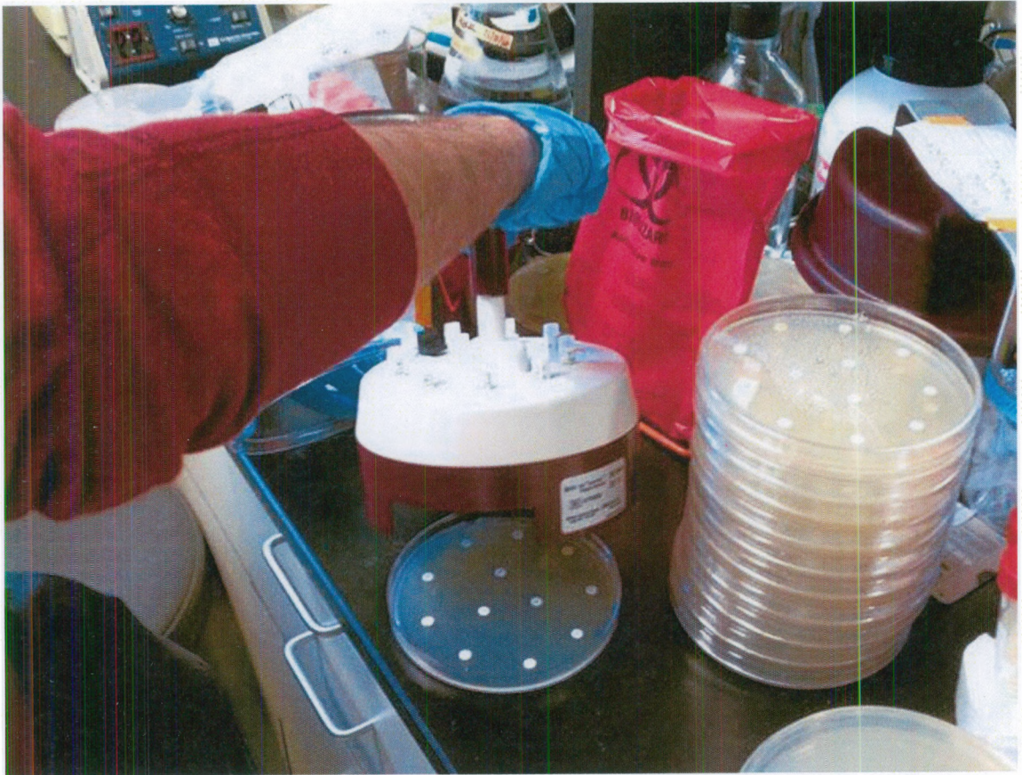
Figure A.2: Kirby-Bauer Method for Antibiotic Disk Diffusion Testing
