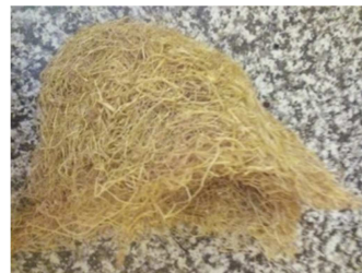
Fig. 5 Sodium hydroxide treated maize stalk cellulose fibers
