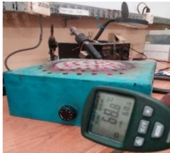
Fig. 8 Heat level measurement on the proposed electric stove
