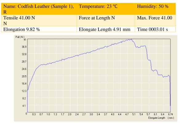
Table 1. Present the results of measurements performed according to ISO 6943:2003, sample
