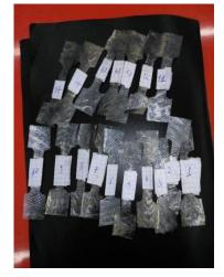
Figure 2. Shape of the fish test pieces for tensile testing
