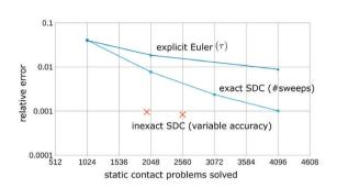
**Figure 5:** Efficiency of different time integrators for long-time wear simulation on 200 000 load cycles. The computational effort is measured by the number of static contact problems to be solved.
