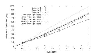
**Figure 4:** Total wear mass loss as a function of time for different cycle jumping step sizes.
