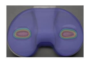
**Figure 3:** Overlay of simulated and experimental wear after 5 million gait cycles.
