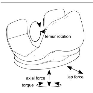
Figure 2: Load directions of the ISO 14243 standard.
