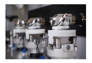
Figure 1: Hardware wear testing of knee implants. The femoral (upper) components undergo a prescribed motion for one to five million load cycles, after which the total wear is determined by the loss of mass in the tibial (lower) part.
