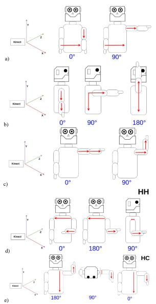
Fig. 5. Vectors used to compute: a) Shoulder opening; b) shoulder rotation; c) Elbow opening; d) Elbow opening with shoulder low; e) Elbow opening with shoulder high
