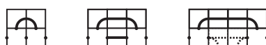
Figure 11. Tiles that share connection points with caps must have four connection points.
