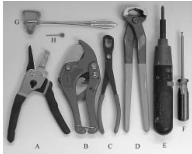
Figure 8. Helmet removal tools. A, facemask extractor; B, PVC pipe cutter; C, Trainer's Angel; D, wire cutter; E, electric screwdriver; F, manual screwdriver; G, reflex hammer (used to pry away cheek pads); H, air pump needle (used to deflate the helmet air bladder). (Anvil pruner and 18-gauge needle not pictured.)
