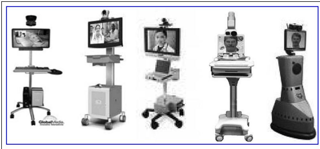
Fig. 7. Portable devices to include (from left to right) Global Media cart, Polycom cart, Tandberg cart, Intouch Health cart, and Intouch Health “Robot.” All the devices just described are dependent on local personnel for movement except the “Semi-Autonomous” Intouch Health robot on the far right.
