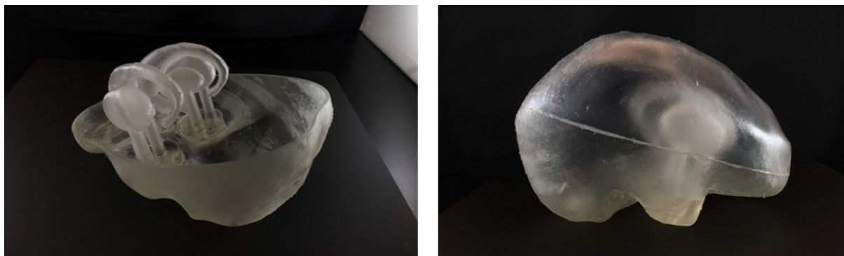
Figure 4.1: Printed brain phantom
