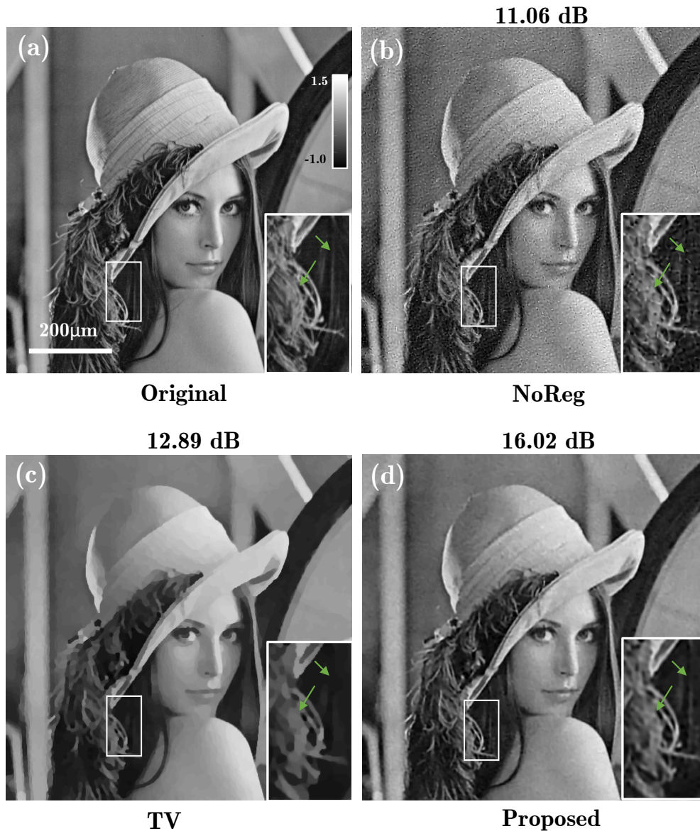
Figure 3.1: Comparison of reconstruction results for Lenna from 16 measurements. (a) shows the original images. (b), (c), and (d) present results using no regularization (NoReg), TV regularization (TV) and proposed regularization (Proposed), respectively. Each image is labeled with its SNR value with respect to the original image.
