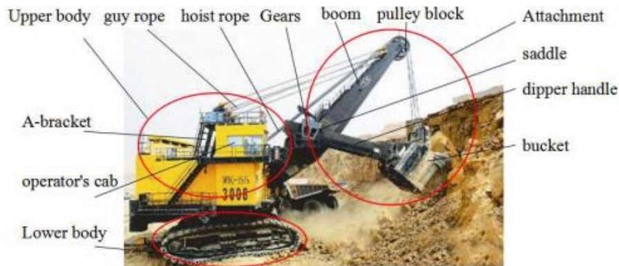
Fig. 1 The system composition of a typical large-scale excavator
