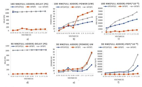
**Fig. 10** (a) Delay, (b) Power, (c) PDP [180nm] and (d) Delay, (e) Power, (f) PDP [90nm] comparison utilizing different supply voltages 0.5V-1.2V
