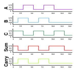
Fig. 9 Input-output waveforms for the proposed FA circuit
