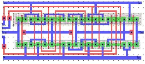
Fig. 8 Proposed FA circuit in Microwind
