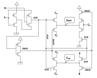
Fig. 5 Proposed Full Adder circuit
