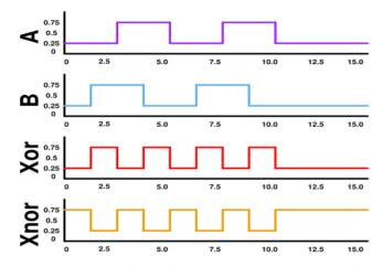
Fig. 7 Input-output waveforms for the proposed XOR-XNOR circuit
