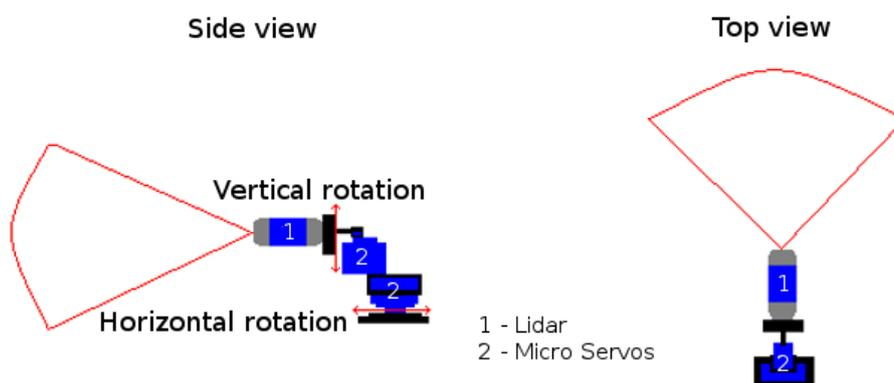
Figure 3. LIDAR rotation.
