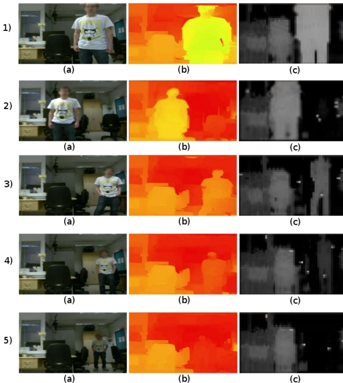
**Figure 8. Results. (a) original image, (b) disparity map (Passive Vision), (c) point cloud map (Active Vision).**
