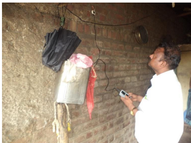
Photo 2: Data backup from the loggers
