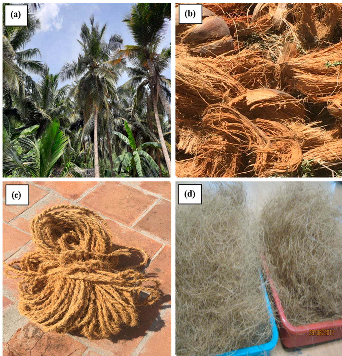
Fig. 11. (a) The coconut tree (b) Coir fibres; from the outer layer (husk) of the coconut (c) Rope made from the coconut fibre (d) Technical coir fibres.
