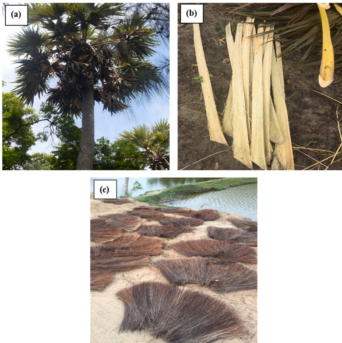
Fig. 13. (a) The Palm tree (b) Palm fibres from the leaf stalk (c) Palm fibres from the leaf base.
