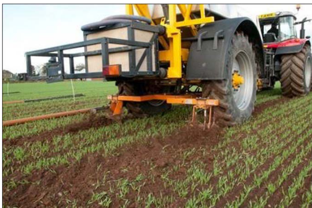
Figure 5. Photograph of rotary harrow in operation. Note; the block of concrete is to provide the same weight as the spray equipment (courtesy of B. McKenzie).
