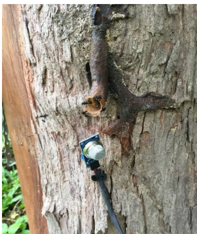
Figure 5. Gas Sensor attached near at the funnel of stingless beehive
