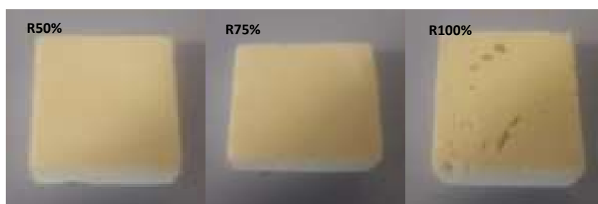
Figure 7. Internal appearance of the rigid PU foams synthesized with different proportions of the recovered polyols a) from conventional rigid PU foam scraps b) from rigid PU foam scraps containing PCMs.
