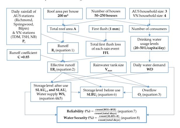
Figure 4. MATLAB modelling input and output parameters for reliability analysis.
