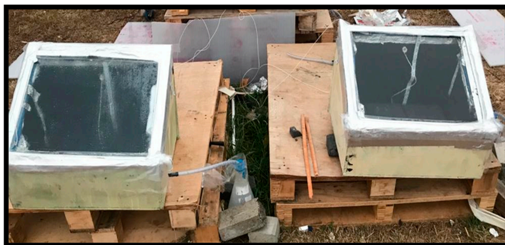
Figure 2. Experimental setup of con-still (left) and mod-still (right).
