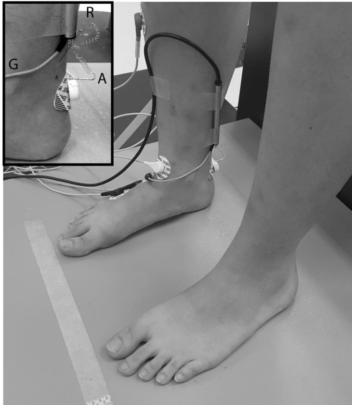
Figure 2.1: Photograph of the experimental set-up. The inset shows a close-up of the electrodes: A = active microelectrode, R = reference microelectrode, G = ground electrode.
