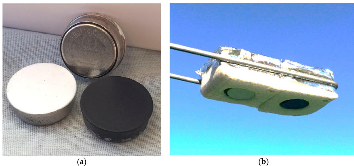
Figure 1. (a) Black- and white-painted iButtons showing the top and back (unpainted) surfaces; and (b) iButtons inset into polystyrene blocks with the upwards facing surface covered in aluminium foil.
