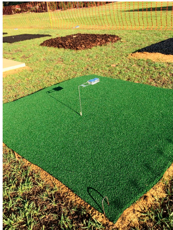
Figure 4. iButtons in their polystyrene casing suspended on a thin metal rod above the centre of the artificial grass. The edges of the 50-mm-thick sand layer are visible.
