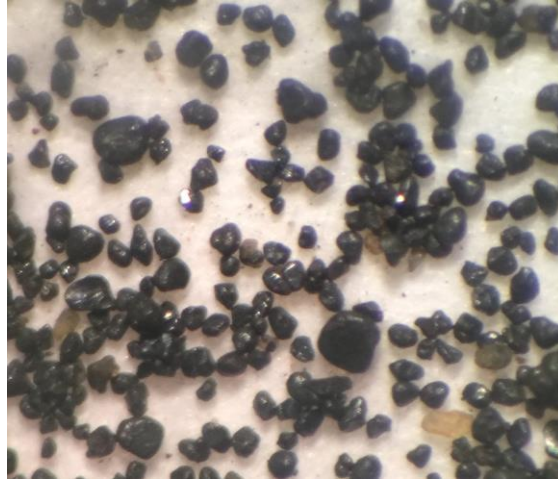
Figure 5.3 Microscopic images for the Black Sand
