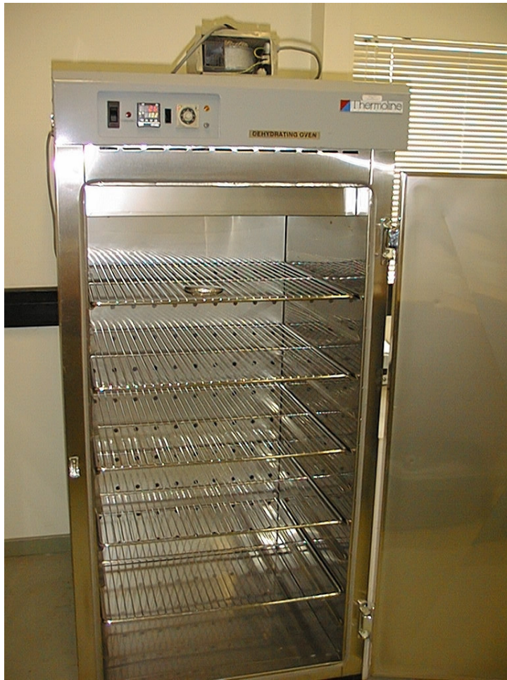
Fig IV. 10 Fan-forced dehydrating oven for drying filter papers and for moisture content measurement
