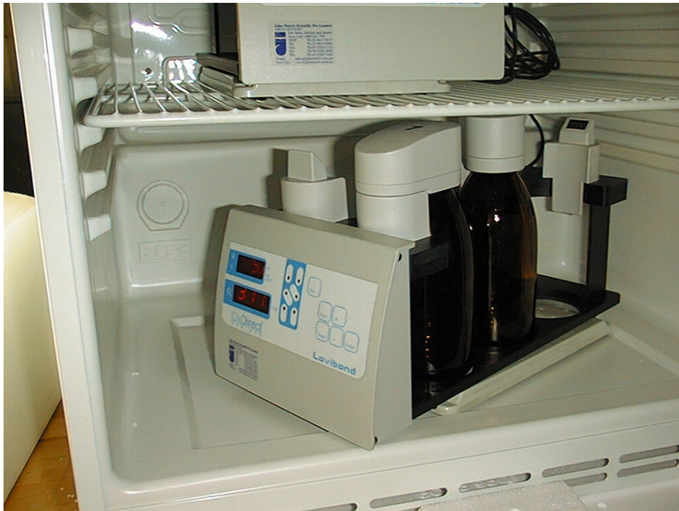
Fig IV. 6 BOD 5 measurement using Oxidirect units
