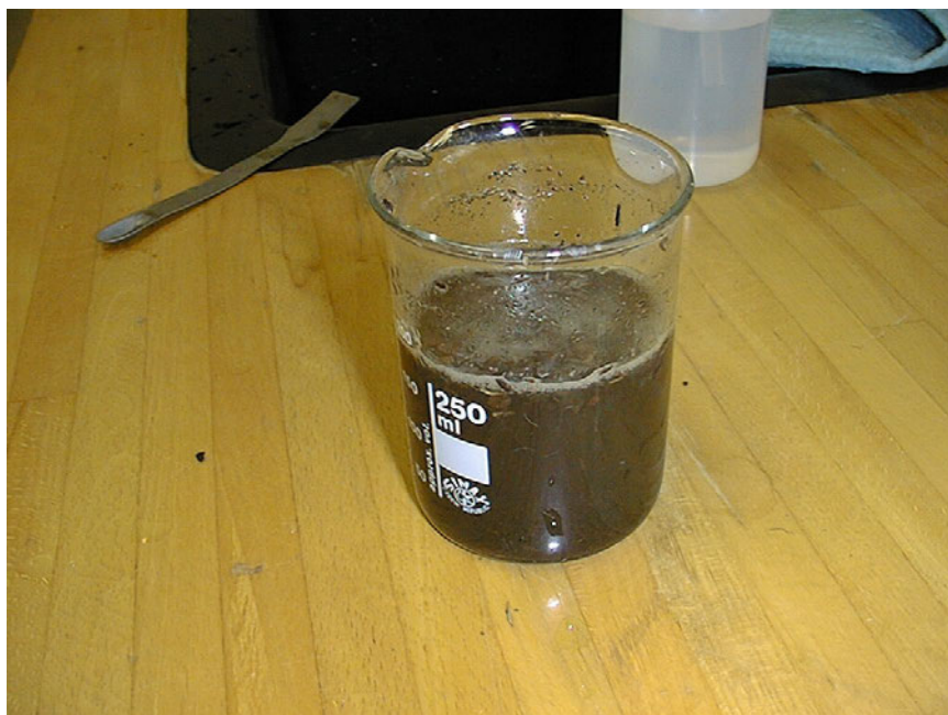
Fig IV.12 Vermicasts in water for extraction – measurements on solids according to Australian Standard AS4454-2003
