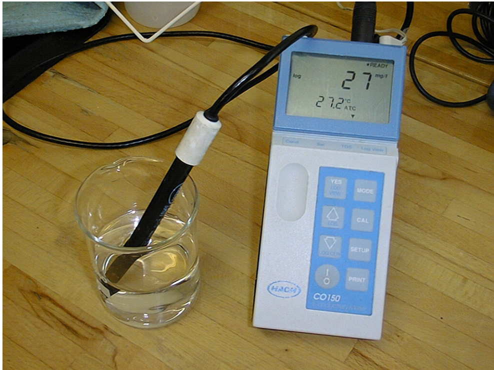
Fig IV.3 Conductivity and TDS measurement using HACH instrument
