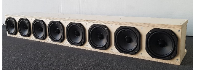
Fig. 10. The 8-channels sound bar of the Wave Field Synthesis system over A 2 B.
