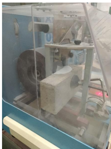
Figure 8. Wide wheel abrasion test on concrete paving blocks.
