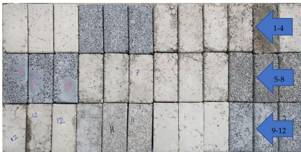
Figure 3. Concrete paving block specimen. Each set of blocks contains 3 repeats and are numbered from right to left. The mixture design of each block is presented in Table 4.
