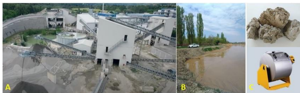
Figure 1. Obtained silt from sedimentation lakes. During aggregate production (A) the produced silt is pumped to the sedimentation lakes (B). The material is oven dried and finely crushed prior to final use (C).
