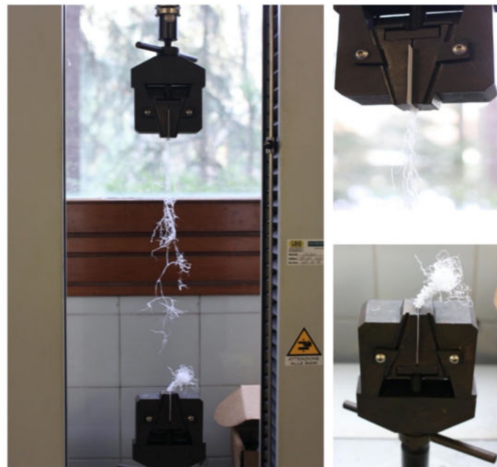
Figure 6. Typical tensile failure of the composite.
