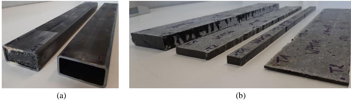
Figure 1. Test specimens: (a) concrete-filled and hollow steel beams; (b) polymer concrete beams.
