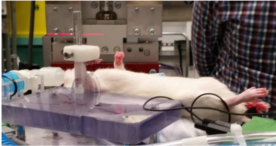
Figure A.2. Three-point contact holder. Photograph showing the three-point contact holder system to limit movement in the limb during scans. The top plate and clear plastic tubing were adjustable for each rat.
