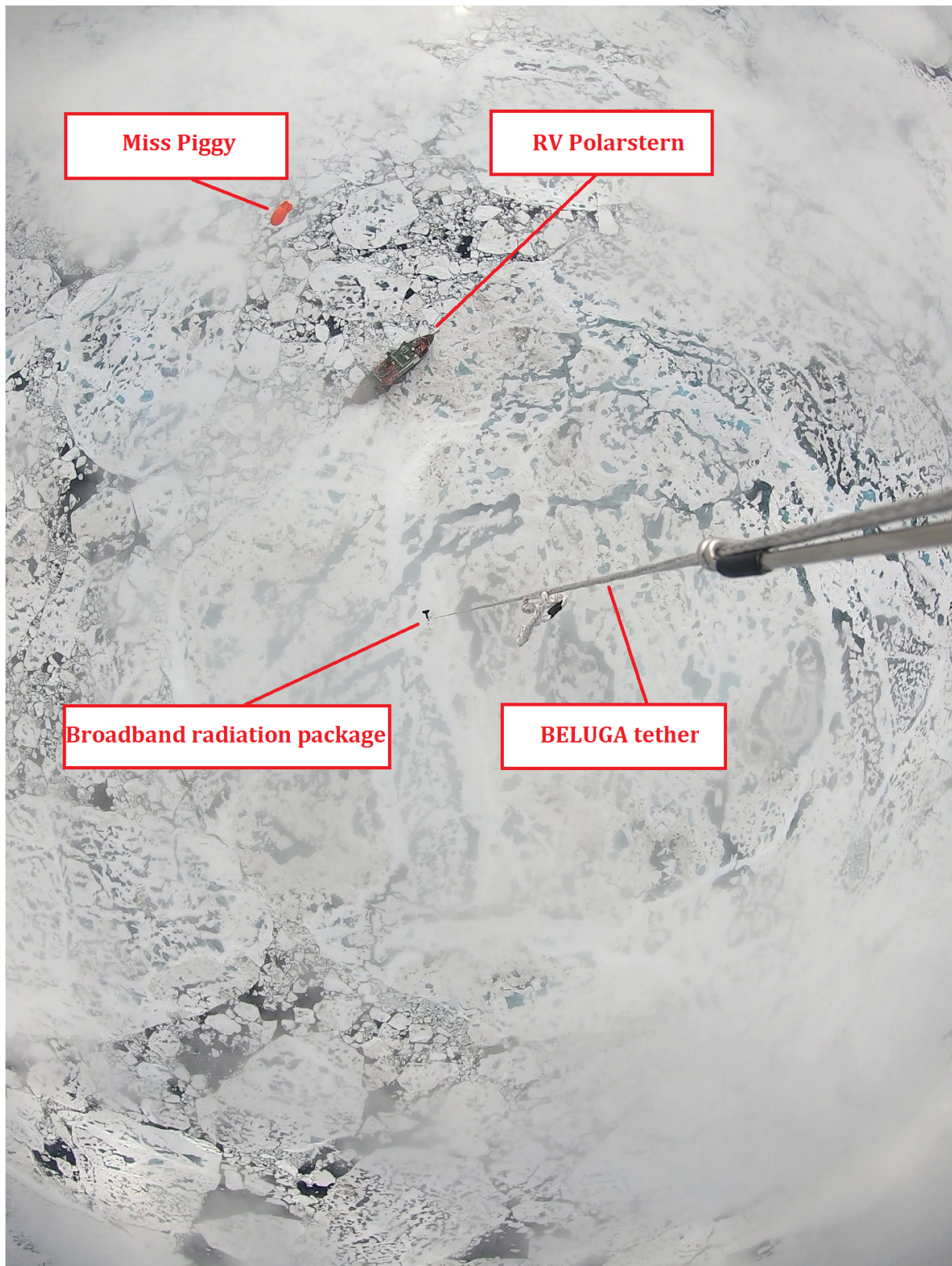
Figure 1: Aerial view of MOSAiC. RV Polarstern, Miss Piggy balloon and the MOSAiC ice floe seen by a camera on BELUGA from about 600 m.
