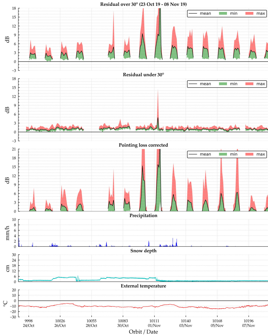
Figure A.22: Residuals and pointing loss comparison against weather effects for cycle 44
