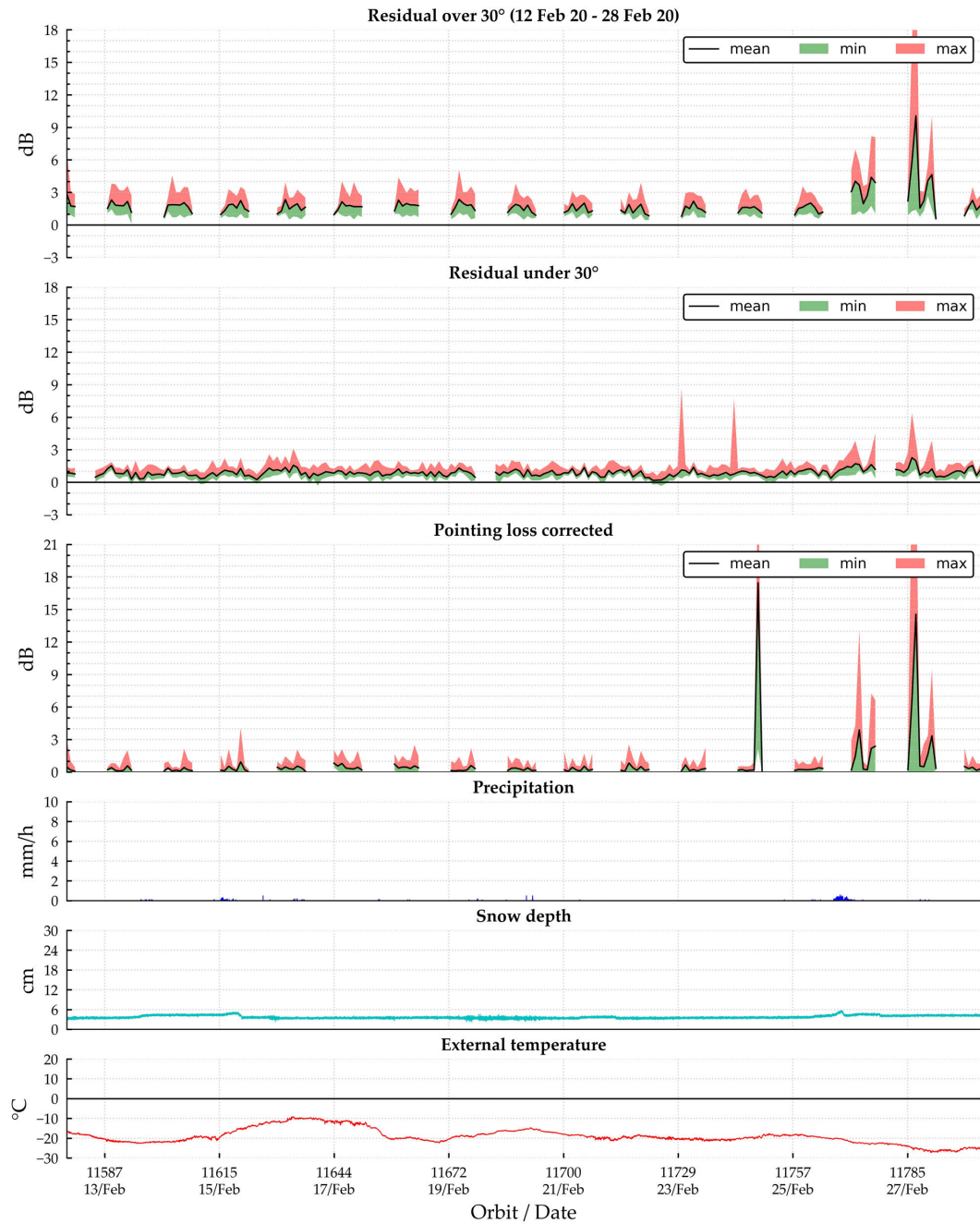
Figure A.29: Residuals and pointing loss comparison against weather effects for cycle 51
