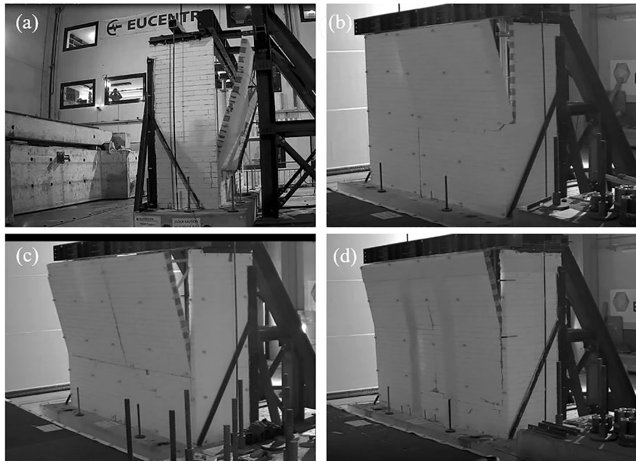
Fig. 2. One-way bending behaviour experimentally observed for Weak Unit-Strong Joint (line failure) URM walls after the exceedance of their peak cracking resistance (PCR): (a) wall CS-000-RF in Graziotti et al. [46]; (b) CS-000-L2; (c) CS-000-RFV and (d) CS-000-RF2 in Sharma et al. [47].
