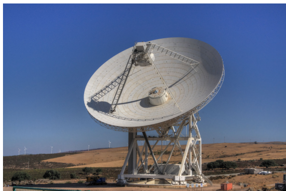
Figure 5.1: Picture of the Sardinia Radio Telescope, example of a deep space antenna employing mechanical beam steering
