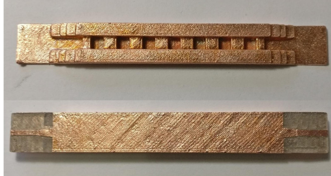
Figure A.9: Prototype of the Bragg reflector bandpass filter
